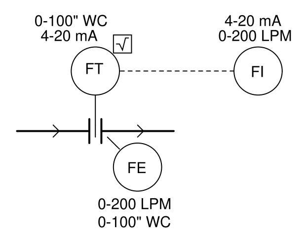
Note that the transmitter is equipped with internal square root characterization, so that no external square root computer is required.
