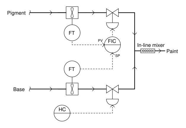
After a couple of years of successful operation, the system begins to output paint that is "paler" in color than it should be. Identify the likelihood of each specified fault for this control system. Consider each fault one at a time (i.e. no coincidental faults), determining whether or not each fault could independently account for the pale-colored paint.
