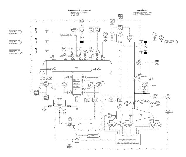
Flowmeter FT-75 has been in service for many years, but unfortunately does not provide good enough turndown for operations' needs when the compressor is operated at a fraction of its rated capacity. Engineers are debating what type(s) of flowmeter might be used to replace FT-75.
