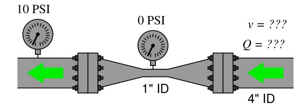
The inside diameter (ID) of the throat is 1 inch, while the inside diameter of the wide pipe is 4 inches. Assume the fluid to be water ( $\rho = 1.94 \text{ slugs/ft}^3$ ) at a constant downstream pressure of 10 PSIG:
