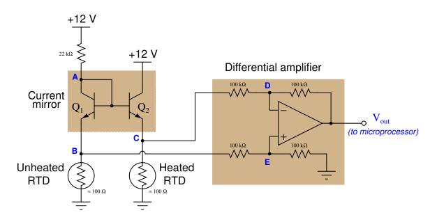
A *current mirror* works to keep current through both RTDs equal, while a differential amplifier measures the difference in voltage drops across the two RTDs.
