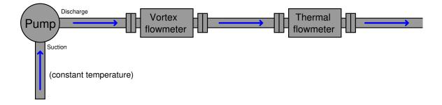
Suppose the positive displacement pump continues to turn at a constant speed, with the temperature of the incoming liquid constant. Suddenly, a steam pipe located near the pump breaks open, directing hot steam at the discharge pipe of the pump, heating the fluid as it exits the pump.
