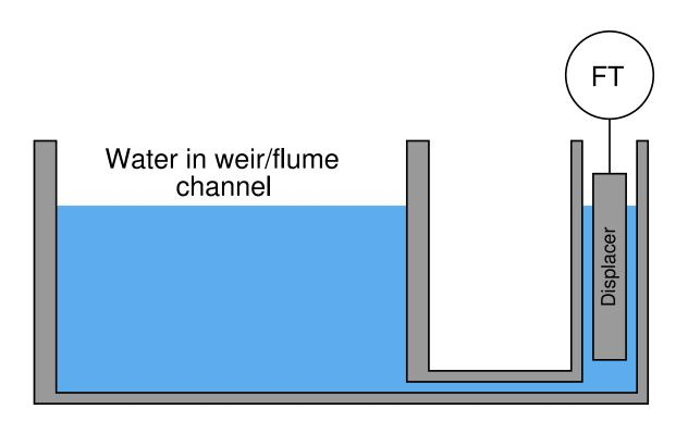
This level-sensing instrument usually provides the characterization necessary to linearize the weir or flume's nonlinear flow/height response. If the level-sensing instrument is ultrasonic, the flow characterization may be done in the same digital computer that calculates liquid level by timing the sound echoes.
