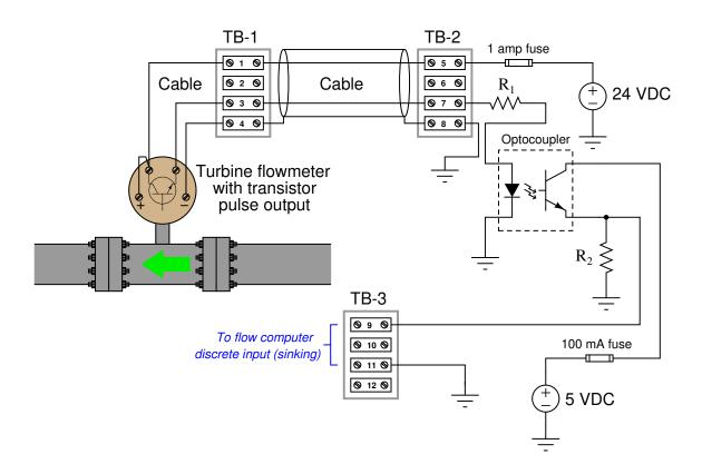
Determine the diagnostic value of each of the following tests. Assume only one fault in the system, including any single component or any single wire/cable/tube connecting components together. If a proposed test could provide new information to help you identify the location and/or nature of the one fault, mark "yes." Otherwise, if a proposed test would not reveal anything relevant to identifying the fault (already discernible from the measurements and symptoms given so far), mark "no."
