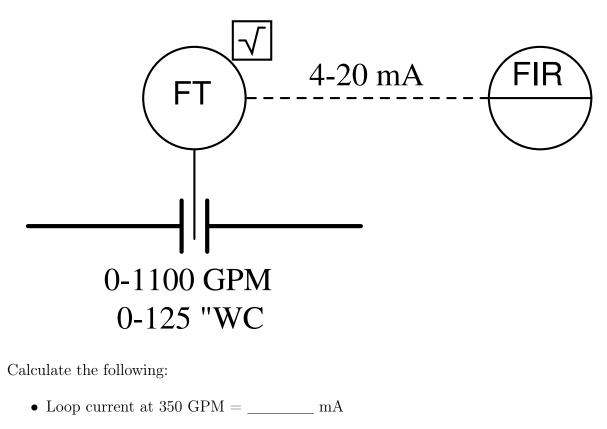
• Differential pressure at 600 GPM = \_\_\_\_\_ "WC
