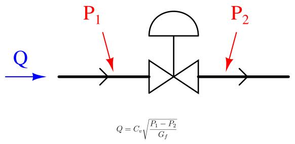
The variable  $C_v$  is called the *flow coefficient* of the control valve, and it varies from zero at full-closed to a certain maximum value (depending on valve size and type) at wide-open.
