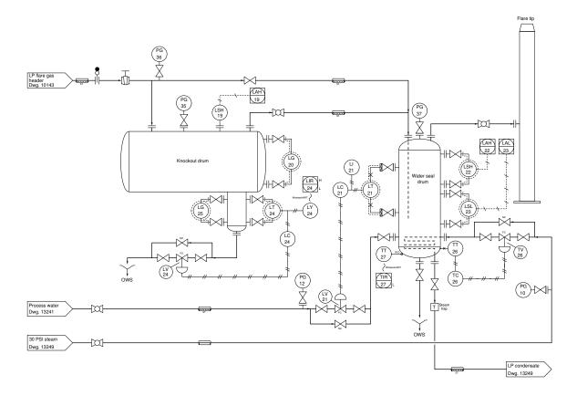
As with most flare systems, the exact composition of material sent to the flare to be burned is both highly variable and unknown from moment to moment. In a typical refinery, anything from hydrogen gas to diesel fuel might get sent to the flare during a "depressurization" event.
