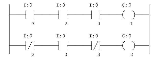
Suppose we have an Allen-Bradley MicroLogix 1000 controller connected to three push-button switches as shown in this illustration:
