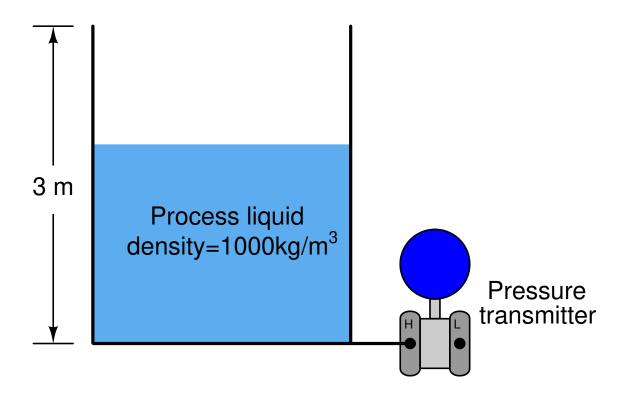
Later, a top is added to this vessel to keep rain from entering in. Unfortunately, though, this process liquid tends to emit vapor which will be trapped by the closed vessel and create a pressure inside of it. A small vent is added to the top of the vessel to permit the vapor to escape, but it is a *small* vent, not big enough to ensure a total absence of vapor pressure buildup at all times:
