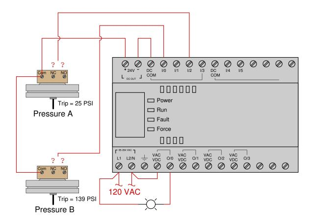
Determine the necessary contacts on each pressure switch (NO versus NC) we need to connect to the PLC inputs in order to make the lamp turn on when pressure A exceeds 25 PSI and pressure B drops below 139 PSI, given the following program running in the PLC:
