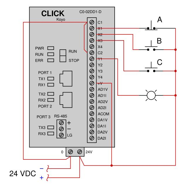
Sketch a Ladder Diagram program for this PLC to energize the lamp if the following input conditions are met:
