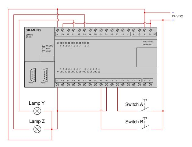
Examine the following relay ladder logic (RLL) program for this Siemens PLC, determining the statuses of the two lamps provided both switches are simultaneously pressed by a human operator:
