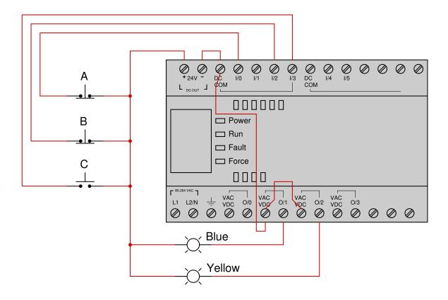
Determine the necessary switch actuation statuses (i.e. pressed versus unpressed) to turn the blue lamp on, given the following program running in the PLC:
