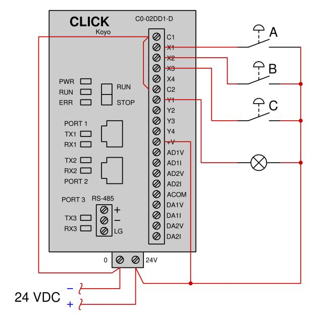
Determine the switch actuation statuses (i.e. pressed versus released) given the "live" display of the ladder logic program shown here:
