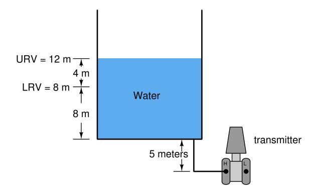
Assuming a pneumatic transmitter with an output range of 4 mA to 20 mA, and a calibration accuracy of +/- 1% of span, complete the following calibration table for the transmitter:
