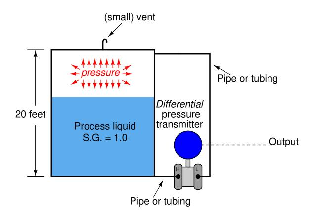
Because the differential pressure transmitter solution requires only one sensing instrument rather than two, and results in better accuracy because we are only dealing with
