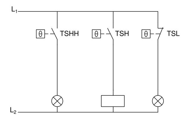
Temp. high Cooling water Temp. low solenoid
