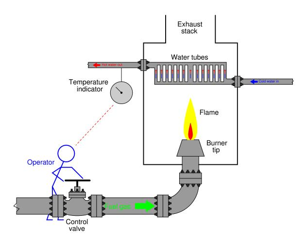
Does the operator play the part of a *direct-acting* controller, or a *reverse-acting* controller, in this process control scenario?
