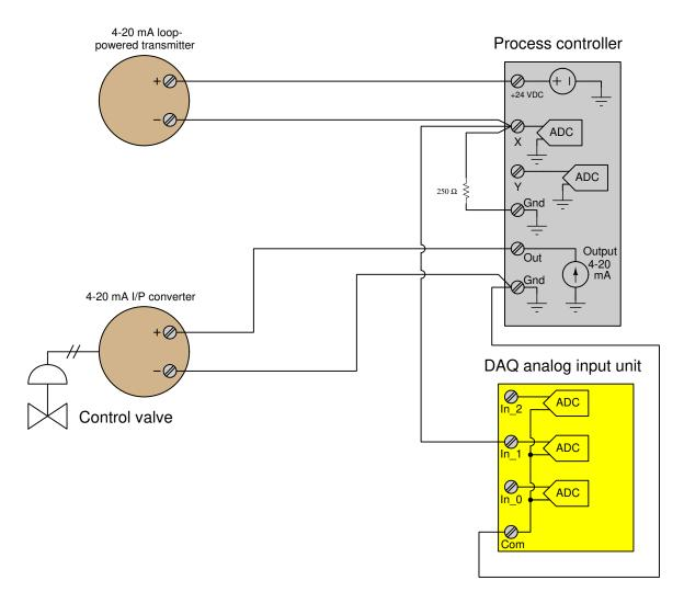
Unfortunately, the DAQ not only registers the DC signal value, but also any HART pulses present in the transmitter circuit whenever a technician connects a HART communicator to the transmitter to do any maintenance work. The operators are annoyed by the misleading "noise" on the DAQ-recorded signal whenever a technician does routine work on that transmitter, and so they come to you asking for a solution.
