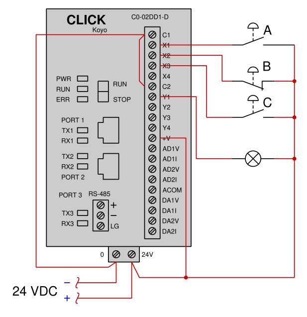
Determine the necessary switch actuation statuses (i.e. pressed versus unpressed) to turn the lamp on given the following program running in the PLC:
