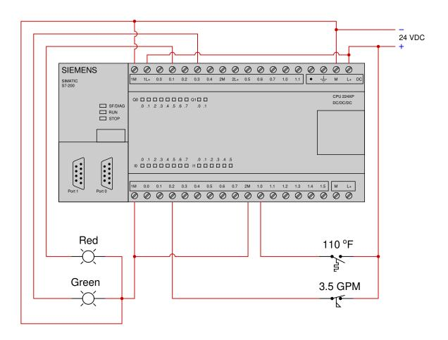
Examine the following relay ladder logic (RLL) program for this Siemens PLC, determining the statuses of the two lamps provided the temperature switch senses 102  $^o\mathrm{F}$  and the flow switch senses 4.7 GPM:
