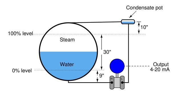
Assume a density for (hot) boiler drum water of  $36 \text{ lb/ft}^3$ , a density for steam in the drum of  $7 \text{ lb/ft}^3$ , and a density for (warm) water in the "wet leg" of  $61.8 \text{ lb/ft}^3$ . If the pressure at the "low" (L) side of the transmitter is greater than the pressure at the "high" (H) side, be sure to express the differential pressure quantity as a negative number.
