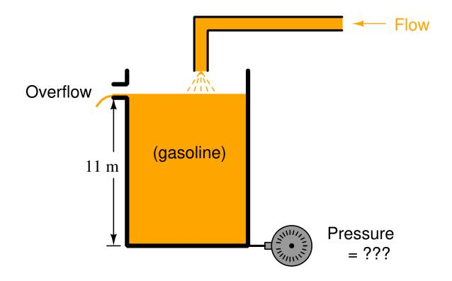
What do you think the pressure will be at the bottom of the vessel if it is exactly half-full of gasoline and half-full of water, with a gasoline-water *interface* at the 5.5 meters mark? Explain your reasoning.
