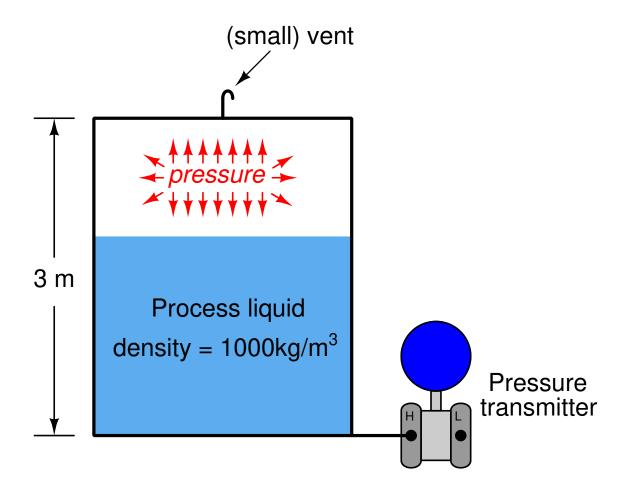
What problem in level measurement will result from there being an occasional vapor pressure buildup inside this vessel? How may this problem be corrected so that the liquid level will be accurately measured at all times?  $\frac{1}{100248}$
