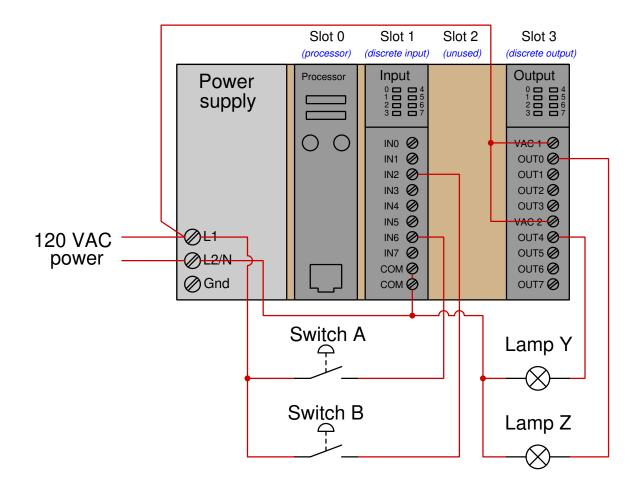
Examine the following relay ladder logic (RLL) program for this Allen-Bradley PLC, determining the necessary switch statuses to energize lamp Y, and the necessary switch statuses to energize switch Z:
