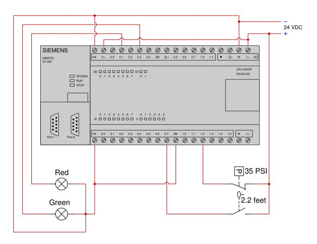
Examine the following relay ladder logic (RLL) program for this Siemens PLC, determining the statuses of the two lamps provided the pressure switch sees a fluid pressure of 30 PSI and the level switch sees a liquid level of 4 feet:
