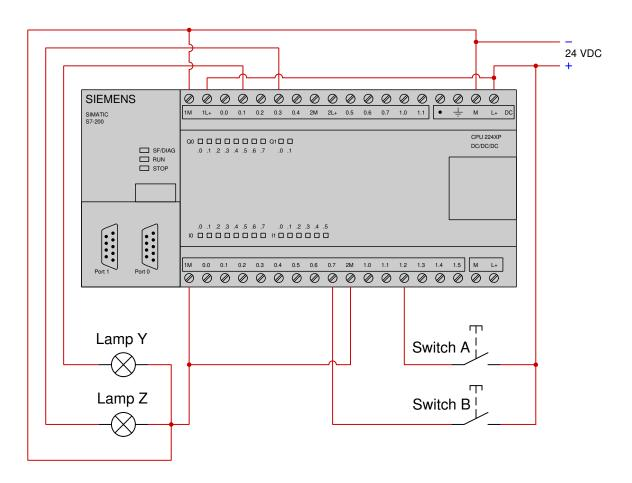
Examine the following relay ladder logic (RLL) program for this Siemens PLC, determining the statuses of the two lamps provided neither switch is pressed by a human operator:
