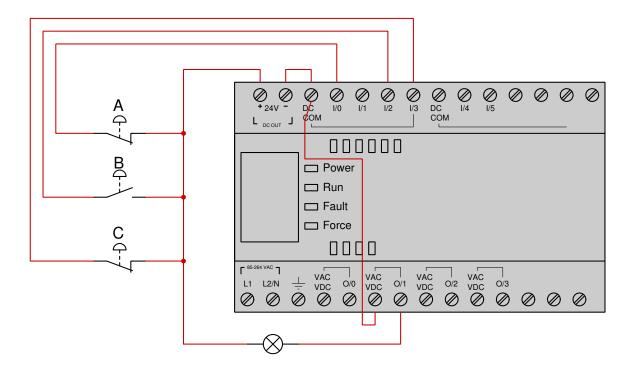
Determine the necessary switch actuation statuses (i.e. pressed versus unpressed) to turn the lamp on given the following program running in the PLC:
