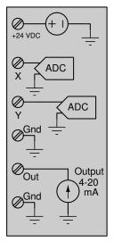
Show how all three field devices would properly connect to the controller, including the placement of resistors to convert the current signals into voltage signals that the controller's ADC's may interpret. Furthermore, use shielded cable, showing where all shield ground connections should be located.
