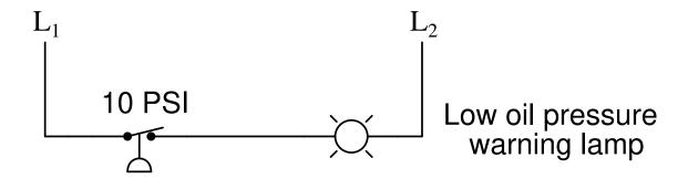
As the diagram shows, this needs to be a **normally-closed** switch.
