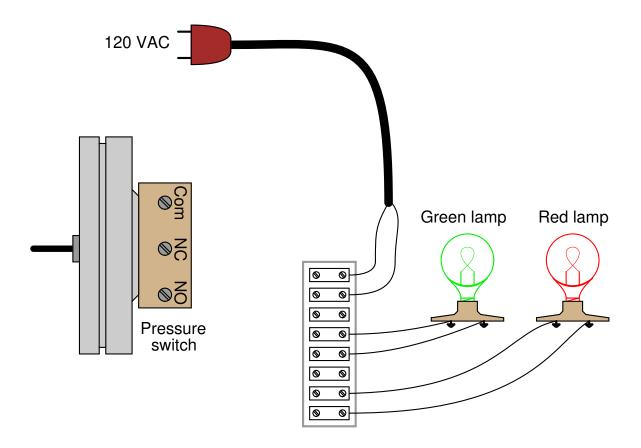
Hint: remember that the "normal" status of a switch is defined as the status of *minimum stimulus*: when the switch is exposed to the lowest possible degree of process stimulation (in this particular case, to the lowest possible pressure). file i03251
