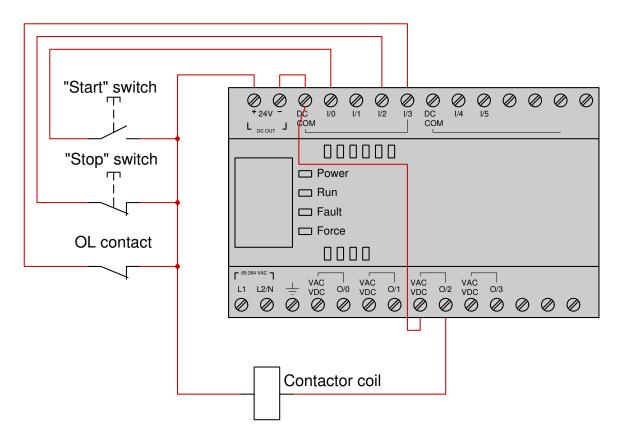
This motor control system has a problem, though: the motor refuses to start when the "Start" pushbutton is pressed. Examine the "live" display of the ladder logic program inside this Allen-Bradley PLC to determine what the problem is:
