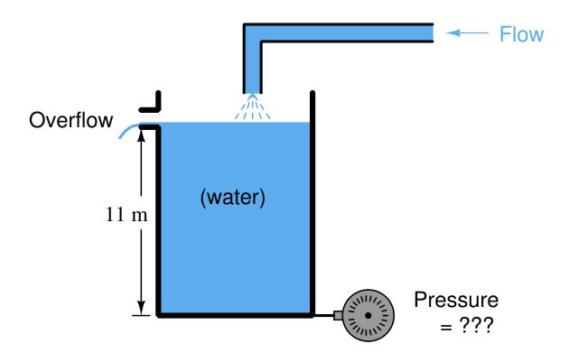
Now calculate the hydrostatic pressure at the bottom of this vessel (in units of bar) when it is completely filled with gasoline (density =  $672.8 \text{ kg/m}^3$ ):
